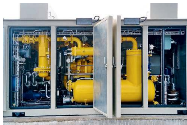
PHOTO 4. Gas compressor equipment as a part of UEC-UMPO PJSC test bench
